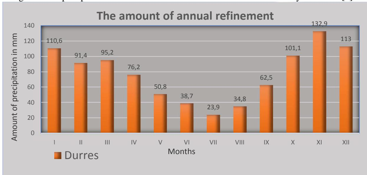
The shape and the roof footprint play an important role in determining the amount of precipitation. For 100 m<sup>2</sup> of roof, 1 – 2 litres of water are obtained in a min (in our calculations we will consider an average value of 1.5 l/min). For 24 hours are obtained: 1440 min x 1.5 l/min = 2 160 l/day of water. Total number of rainfall days 116 days x 2 160 l = 250 560 litres of water in a year [1].
